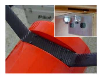
2. Install the landing gear axles with lock nut, but do not tighten
