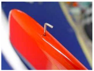
3. Tighten the collar set screw with 1.5mm Hex Wrench as shown
