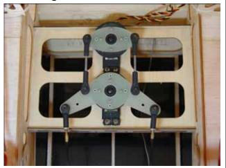
NOTICE: The coupler is best to thread half way into ball link for further tightening next
