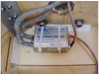
3. Lock the connectors with the provided safety clip against vibration and loosened tension as shown
