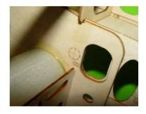
The location of CG has been marked inside plane as show. Usually it is near the wing tube.
