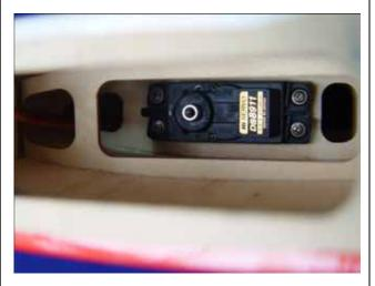
3. Install the servo arm with mounting screw and make it vertical with ground. Adjust pushrod in proper length to keep the aileron panel on the neutral position
