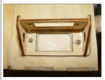
5. Finish the servo installation with mounting screws
