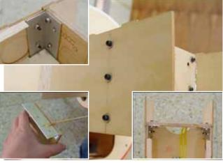
Note: Epoxy the triangular hardwood supports for reinforce.100cc firewall needs to cut off the center hole for air exit
