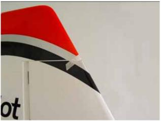
3. Attach the pre-installed boll link to the rudder horns without locking nut as shown
