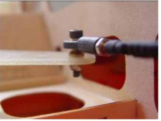
10. Turn off the radio now. Reinstall the ball link (Don't pull strongly to hurt the rudder or back to step 7 for readjustment )you can find a helper and do that at certain deflection with supporting the bottom of the rudder.
