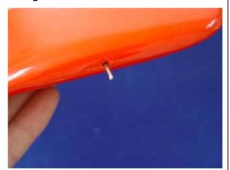
2. Align the rudder in place inserting the steering arm through the steering tube in top of rudder ensure pin bent end sits flush on top of rudder
