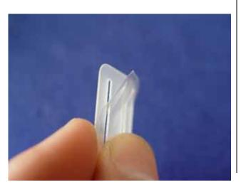
2. Trace around the locking plate with kinfe and cut off the cover below. Then the pre-cut slots appear
