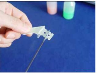
5. Slide the horns into slots slightly and Mount the locking plate in place. Align the right and left sides before epoxy has cured. Wipe away excess epoxy with rubbing alcohol
