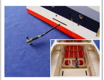
1. Mount servo with mounting screws and face the brand toward the rudder. Drill holes with 1mm bit
