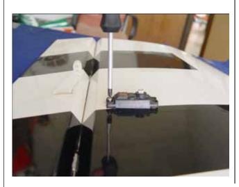
6. Install the servo arms facing toward the wing tip and adjust pushrod in proper length to keep the aileron panel on the neutral position
