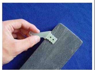
4. Apply the 30 minutes epoxy inside the pre-cut slots, and coat the horn with epoxy as shown
