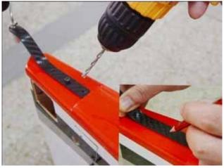
3. Install the blind nuts through the opening in the rear of the fuse and mount screws for the tail wheel using Blue Loctite in the thread
