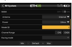
The system will assign you the receiver a number automatically, when you create a new model, and this can be easily changed. The range of the Model ID is 00-63, with the default number being 01. Once the receiver is set to the desired number and is bound to the TANDEM X20 HD, the bind procedure will not need to be repeated unless the receiver number is changed. At this point, set the receiving number to your preferred number and repeat the binding operation
