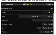
The external RF module can be powered on or off by software. The setup process is the same as that for the internal RF. External modules should be closed when
